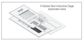
gradients in field intensity, additional measures may be required. For this purpose, Vishay Micro-Measurements has developed a special gage configuration, the H-Series, consisting of two identical grids, with one stacked directly above, and insulated from, the other. By connecting the upper and lower gage elements in series so that the current
