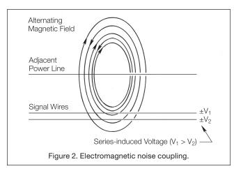
Since most irons and steels are ferro-magnetic, moving machine members redirect existing lines of flux, and may cause them to be cut by adjacent sensitive conductors. As a result, signal conductors in the vicinity of moving or rotating machinery are generally subject to noise voltages from this source.
