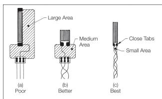
Figure 5. Gage selection and wiring technique.
