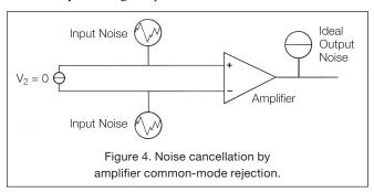
In theory, at least, the more twists per unit conductor length, the better. Standard twisted-conductor cables, such as Belden No. 8771, have sufficient twisting for most applications. However, in environments with high magnetic field gradients, such as those found close to motors, generators, and transformers, tighter twisting may be required. For particularly severe applications, conventional twisting may be inadequate, and it may be necessary to use a special woven cable as described later.
