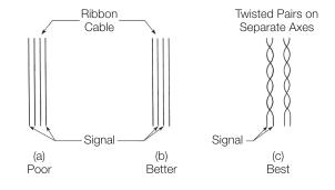
Figure 6. Cable comparison.
